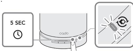
3. Press the timer button again immediately to turn off the filter replacement indicator and complete initialization.
